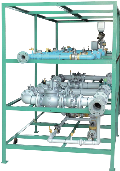
Control devices (Valve stand)
